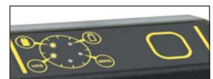
The number of hours is indicated by the number of lit LEDs: 2 LEDs = 2 hours.
