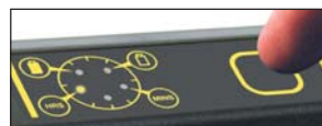
A second button press activates the time display. The 'HRS' LED flashes twice.
