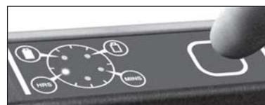
The second button-press activates the time display. The 'HRS' LED will flash twice.
