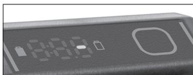
When battery capacity drops below 5% the display will indicate that the battery should be charged by pointing to the empty battery symbol.
