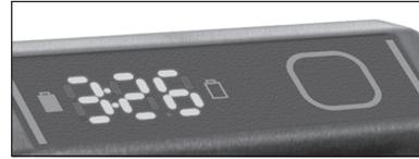
The battery requires a minimum of 5 seconds before it is able to give an accurate run-time prediction.
